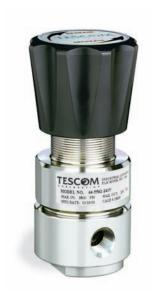
TESCOM 44-5500 Series general purpose, compact backpressure regulator controls pressures up to 300 psig / 20.7 bar and is suitable for gas or liquid service.
