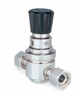
TESCOM 64-3200 Series ultra high purity, high flow tied diaphragm pressure reducing regulator offers 10 R<sub>a</sub> microinch / 0.25 micrometer surface finish and is available in Hastelloy® trim. Maximum flow rates are up to 31.8 SCFM / 900 SLPM, with inlet pressures of 150, 1000, 1500 psig / 10.3, 69.0, 103 bar and outlet pressures up to 200 psig / 13.8 bar.
