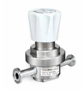
TESCOM PH-2600 Series is part of our Pharmpure™ product line. This high purity single-stage regulator offers a compact, USP Class VI and BPE compliant design suitable for specialty, corrosive, and pyrophoric applications. This regulator offers gas flows of <10 SCFM / 283 SLPM. Diffusion-resistant metal diaphragm seal ensures gas purity and integrity.
