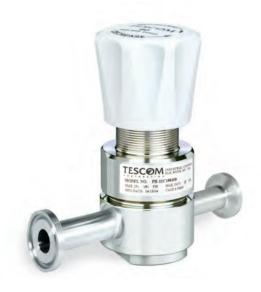
TESCOM PH-2200 Series is part of our Pharmpure<sup>™</sup> product line. This high purity single-stage regulator offers a compact, USP Class VI and BPE compliant design suitable for specialty, corrosive, and pyrophoric gases of < 5 SCFM / 142 SLPM. Diffusion-resistant metal diaphragm seal ensures gas purity and integrity.
