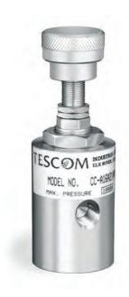
TESCOM CC Series metering valve is rated to 10,000 psiq / 690 bar and contains a non-rotating stem to reduce seat and stem wear. The valve features over 20 turns from shutoff to full open, providing excellent flow control.
