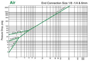
Air Flow S.C.F.M. @ 70°F (21°C) (Discharge to Atmosphere)
