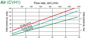
Air Flow S.C.F.M. @ 70°F (21°C) (Discharge to Atmosphere)
