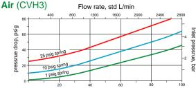
Air Flow S.C.F.M. @ 70°F (21°C) (Discharge to Atmosphere)
