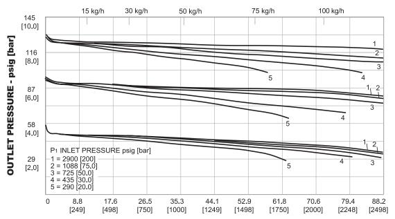
FLOW RATE - SCFM [SLPM] Compressed Natural Gas
