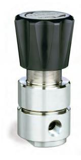
TESCOM 44-2500 Series is a compact, lightweight, single-stage regulator for specialty, flammable, and industrial gases for flows up to 30 SCFM / 850 SLPM. Diffusion-resistant metal diaphragm seal ensures gas purity and integrity.
