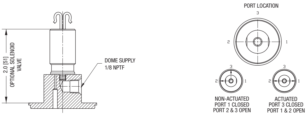
NON-ACTUATED PORT 1 CLOSED, PORT 2 & 3 OPEN
